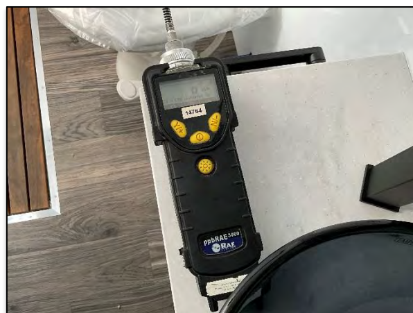
Figure (41) – Trailer #2, Bathroom – VOC monitor reading (0 ppb).
