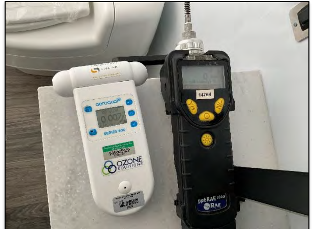
Figure (16) – Trailer #1, Bathroom – Ozone (0.007) and VOC (0 ppb) monitor reading.
