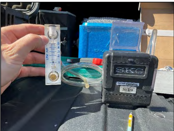
Figure (35) – Trailer #1 – Low volume pump calibration check prior to collection of exterior formaldehyde air sample.
