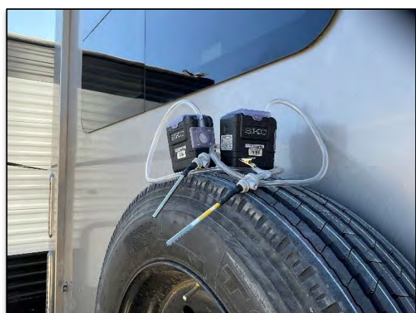
Figure (36) – Trailer #2, Exterior – Formaldehyde air sample (#0044815955).
