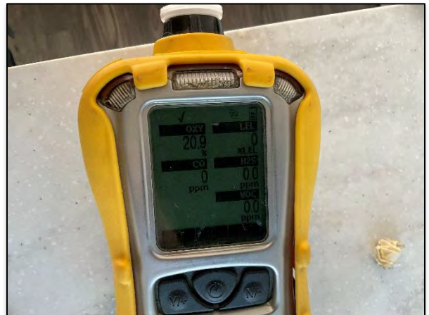
Figure (18) – Trailer #1, Bedroom – 4-gas monitor readings.
