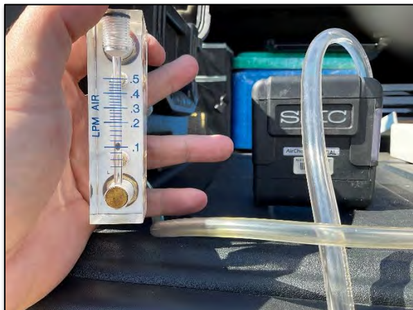
Figure (31) – Trailer #2 - Low volume pump calibrated to 0.1 LPM for exterior TO-17 air sample.
