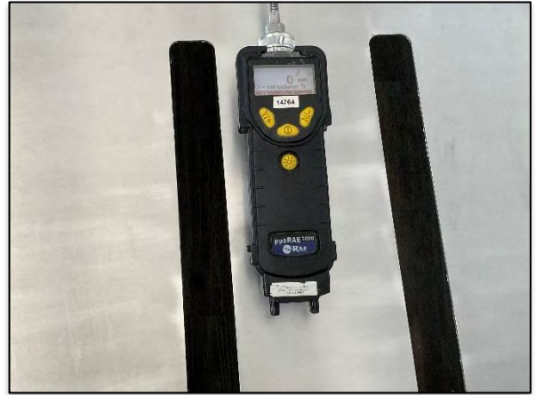
Figure (44) – Trailer #2, Bedroom – VOC monitor reading (0 ppb).
