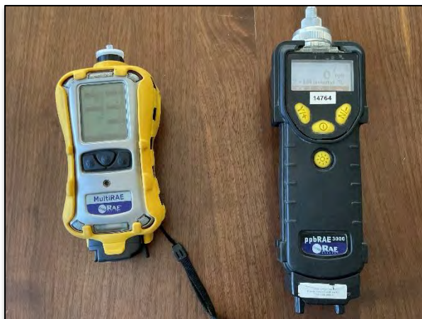
Figure (39) – Trailer #2, Dining Room – 4-gas meter and VOC (0 ppb) monitor reading.
