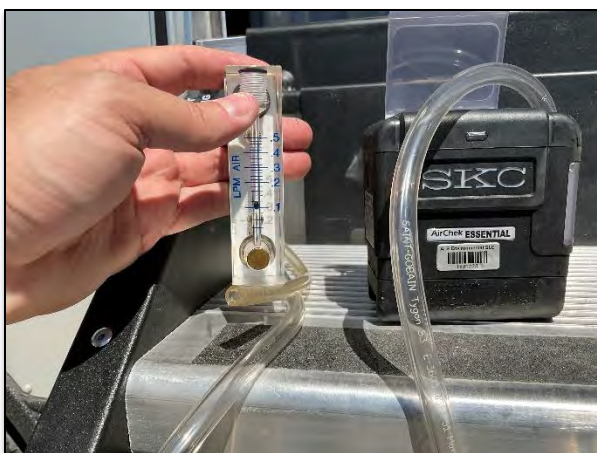
Figure (11) – Trailer #1 – Low volume pump calibration check prior to collection of exterior formaldehyde air sample.
