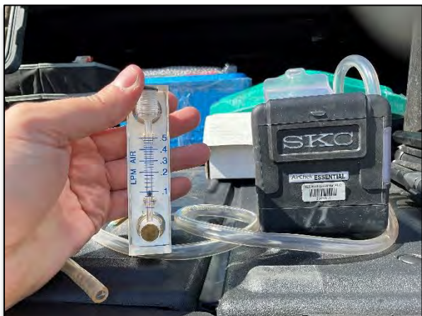
Figure (33) – Trailer #2 – Low volume pump calibration check prior to collection of interior formaldehyde air sample.
