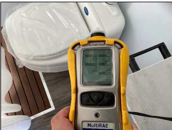
Figure (17) – Trailer #1, Bathroom – 4-gas monitor readings.
