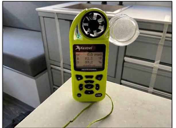
Figure (22) – Trailer #1, Kitchen – Temperature and relative humidity readings.
