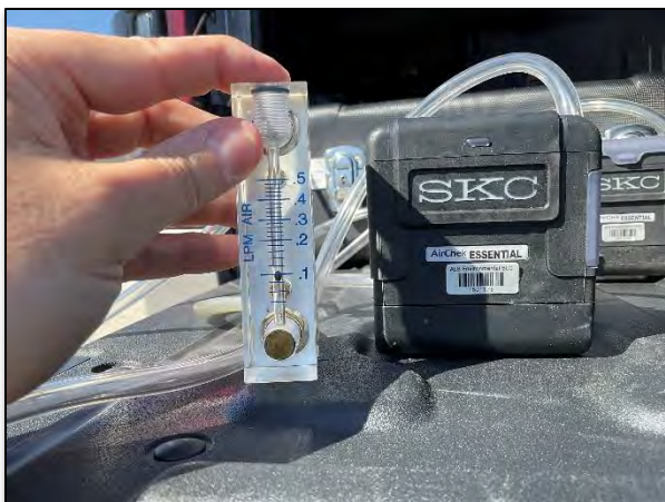
Figure (5) – Trailer #1 – Low volume pump calibrated to 0.1 LPM for interior TO-17 air sample.
