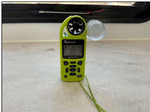
Figure (51) – Trailer #2, Bedroom – Temperature and relative humidity readings.
