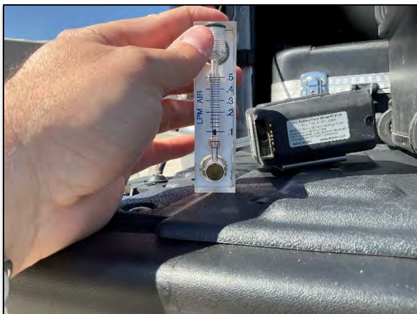
Figure (7) – Trailer #1 - Low volume pump calibrated to 0.1 LPM for exterior TO-17 air sample.
