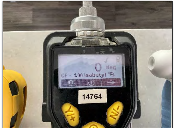
Figure (14) – Trailer #1, Kitchen – VOC monitor reading.
