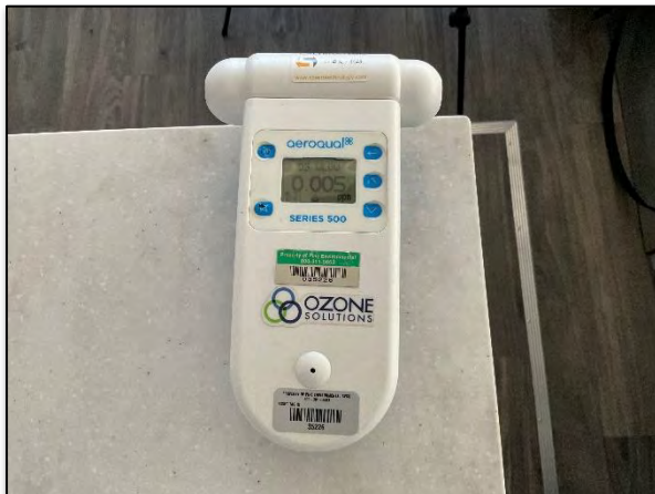
Figure (45) – Trailer #2, Bathroom – Ozone monitor reading (0.005).
