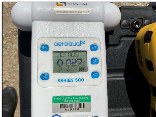
Figure (50) – Trailer #2, Exterior – Ozone monitor reading (0.027).
