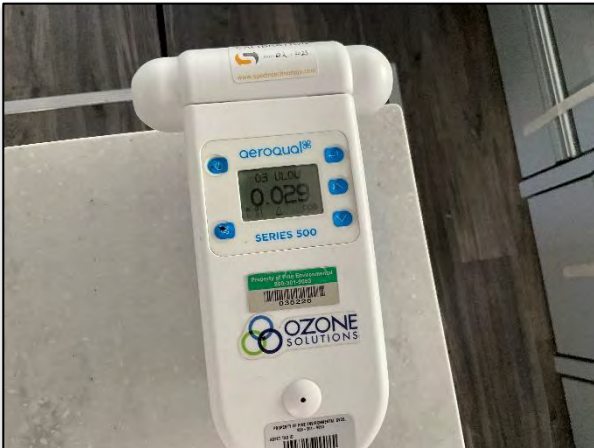
Figure (15) – Trailer #1, Kitchen – Ozone monitor reading.
