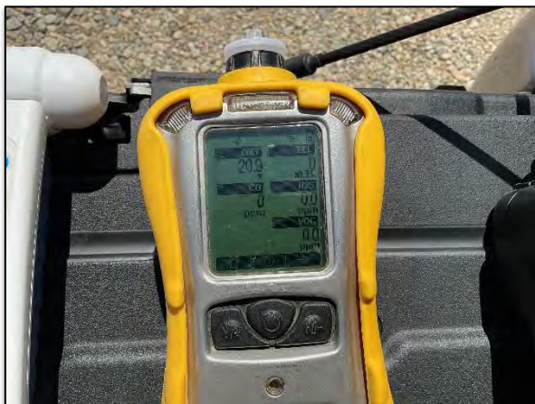
Figure (49) – Trailer #2, Exterior – 4-gas monitor readings.
