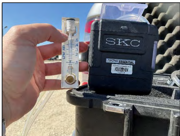
Figure (29) – Trailer #2 - Low volume pump calibrated to 0.1 LPM for interior TO-17 air sample.
